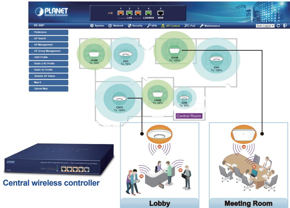
For example, to configure multiple Smart APs of the same model, the VR-300P allows clustering them to a managed group for unified management. According to requirements, wireless APs can be flexibly expanded or removed from a wireless AP group at any time. The AP cluster benefits bulk provision and bulk firmware upgrade through single entry point instead of having to configure settings in each of them separately.
