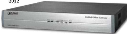
The PLANET UMG-1000 is a desktop total IT solution for the small and medium business (SMB). It integrates commonly used office appliance features and provides Internet access, telephone, fax, data, and print services in one device. Via the built in 4-Port FXO, the UMG-1000 allows SMBs to connect to various Internet and telephone carriers easily.
