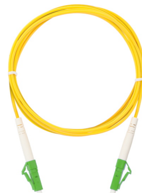
NMF-PC1S2C2-LCA-LCA-xxx SM 9/125 OS2, LC/APC-LC/APC, LSZH, D=2.0mm, Simplex
