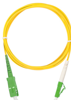
NMF-PC1S2C2-SCA-LCA-xxx SM 9/125 OS2, SC/APC-LC/APC, LSZH, D=2.0mm, Simplex
