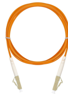
NMF-PC1M2C2-LCU-LCU-xxx MM 50/125 OM2, LC/UPC-LC/UPC, LSZH, D=2.0mm, Simplex
