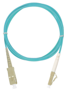
NMF-PC1M3C2-SCU-LCU-xxx MM 50/125 OM3, SC/UPC-LC/ UPC, LSZH, D=2.0mm, Simplex
