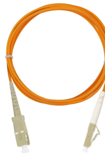
NMF-PC1M2C2-SCU-LCU-xxx MM 50/125 OM2, SC/UPC-LC/UPC, LSZH, D=2.0mm, Simplex
