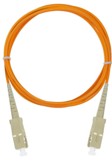
NMF-PC1M2C2-SCU-SCU-xxx MM 50/125 OM2, SC/UPC-SC/ UPC, LSZH, D=2.0mm, Simplex
