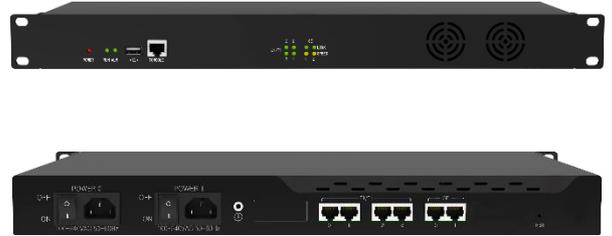
MTG1000 offering PBX/IP-PBX users a powerful telephony cost saving device and advanced flexible routing capabilities between ISDN PRI/SS7 to SIP, and also can be situated between the PBX and the PSTN, saving the cost of an additional PBX E1/T1 port. It is ideal for telecom distributors, resellers and service providers.
